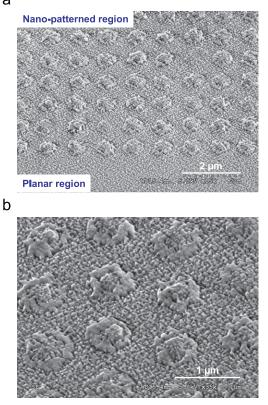
**Fig. 3.** (a) SEM images of nano-patterned and planar sapphire regions with 15 nm GaN buffer layer, and (b) higher magnification SEM image of the nano-patterned sapphire region with 15 nm GaN buffer layer.
