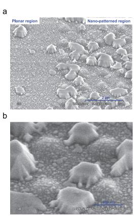
**Fig. 4.** (a) SEM images of nano-patterned and planar sapphire regions with 15 nm GaN buffer layer and 3 min growth of high-temperature GaN, and (b) higher magnification SEM image of the nano-patterned sapphire with 15 nm GaN buffer layer and 3 min growth of high-temperature GaN.
