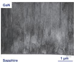
Fig. 7. Cross-sectional TEM images taken at g=(0002) for (a) LEDs sample grown on nano-patterned sapphire with abbreviated growth mode, and (b) LED sample grown on planar sapphire using conventional growth.
