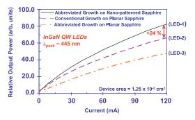
Fig. 6. Room temperature CW light output power as a function of injection current of In<sub>0.15</sub>Ga<sub>0.85</sub>N QW LEDs grown on three comparison templates (LEDs #1, #2, and #3).
