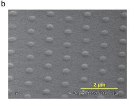
**Fig. 2.** Scanning electron micrographs of (a) aluminum nano-structure array after lift-off, and (b) aluminum nano-structure array conversion to single crystal Al<sub>2</sub>O<sub>3</sub> after two-stage anneal.
