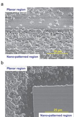
Fig. 5. SEM images of (a) nano-patterned and planar sapphire regions with 15 nm GaN buffer layer and 0.1µm thick high-temperature GaN, and (b) nano-patterned and planar sapphire regions with 15 nm GaN buffer layer and 0.25  $\mu m$  thick high-temperature GaN.
